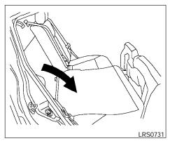
4. Fold down seat backs. See "Interior trunk access (if so equipped)" in this section.
