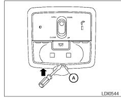
Map light (if so equipped) Use a cloth (A) to protect the light housing.
