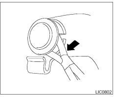
To install the cargo net, attach the net to the retainers.
