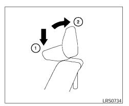
3. To return the head restraint to the normal position, push down ① and release then rotate up until in position ②.
