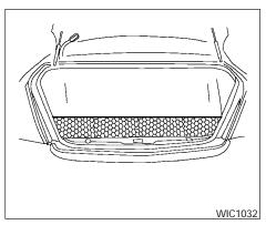
The cargo net helps keep packages in the cargo area from moving around while the vehicle is in motion.
