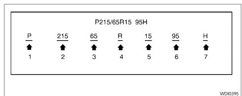
7. H: Tire speed rating. You should not drive the vehicle faster than the tire speed rating.
