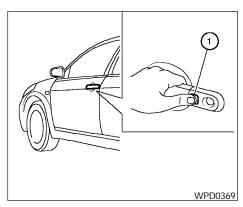
All doors will be locked automatically unless one of the following operations is performed within 1 minute after pushing the request switch.
