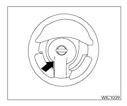
To sound the horn, push the center pad area of the steering wheel.
