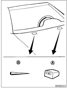
If you wax the surface of the hood, be careful not to let wax get into the washer nozzle (a). This may cause clogging or improper windshield washer operation. If wax gets into the nozzle, remove it with a needle or small pin (a).
