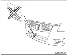
VEHICLE RECOVERY (freeing a stuck vehicle)
