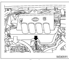
Type A CHECKING ENGINE OIL LEVEL
