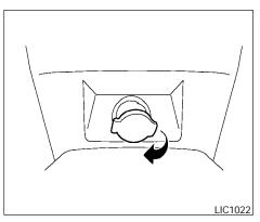
The power outlet is located on the bottom center portion of the instrument panel. The outlet is for powering electrical accessories such as cellular telephones. It is rated at 12 Volt, 120W (10A) maximum.
