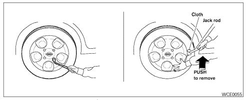
Removing bolt-on wheel cover (if so equipped)
